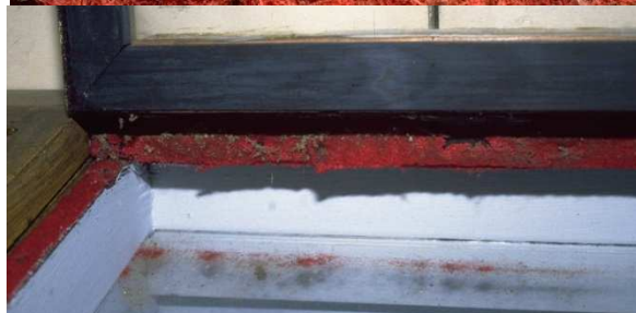
Tineola bisselliella larvae, frass, webs and feeding damage on red wool felt, the dust seal on a display case
